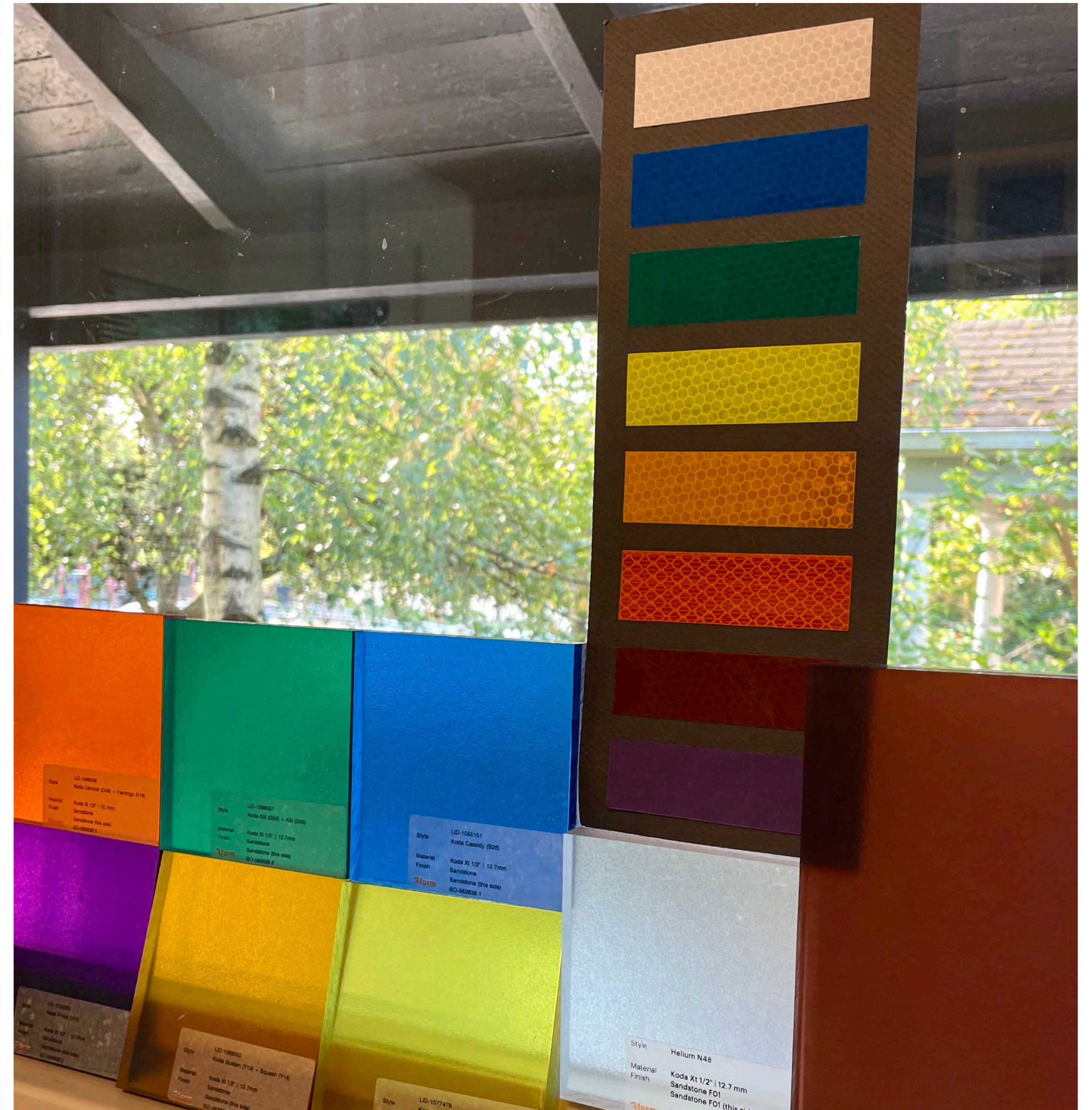
Exterior-rated 1/2"-thick colored polycarbonate (8 colors)
